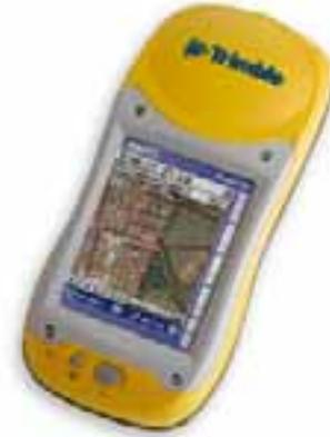
The Trimble GeoXT is a ruggedized handheld computer running the Windows CE operating system. The GeoXT has all-day battery life, two gigabytes of memory, and a built in GPS receiver. It is less sensitive to minor impacts than similar devices and is somewhat water resistant. The GPS receiver has submeter accuracy. The GPS receiver, ability to withstand normal field conditions, and long battery life were all important to creating the desired functionality and high levels of user acceptance.
