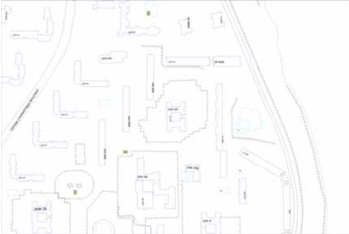
Figure 3: 1:2,000 scale vector data for the Obolon district of Kyiv contains building footprints and is used for municipal mapping and by utilities like Kyivvodokanal. This data is not generally publicly available.
