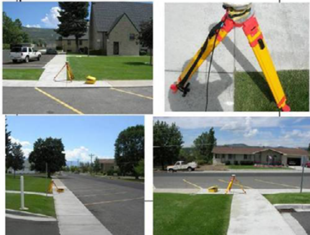
Figure 16: Points were measured and very clearly documented with photos from north, south, east, west, and straight down, in addition to written descriptions.
