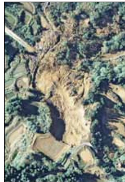
Fig. 9 Flow-type landslides from the ponds probably due to mixing with much water from ponds.
