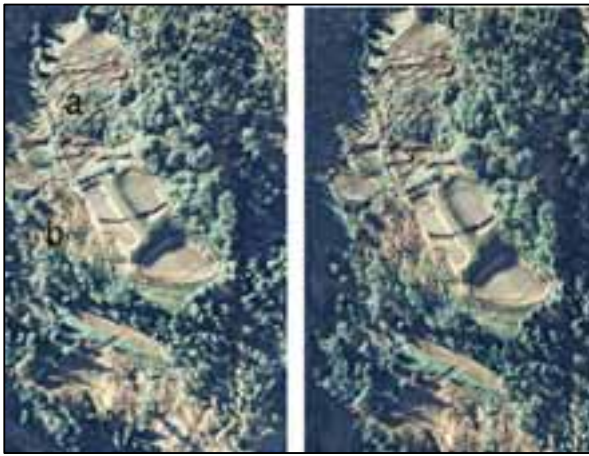
Fig. 8 Stereo-paired photograph showing cracking patterns due to the earthquake. Notice that one (a) is crossing the ponds and the other is arranged
