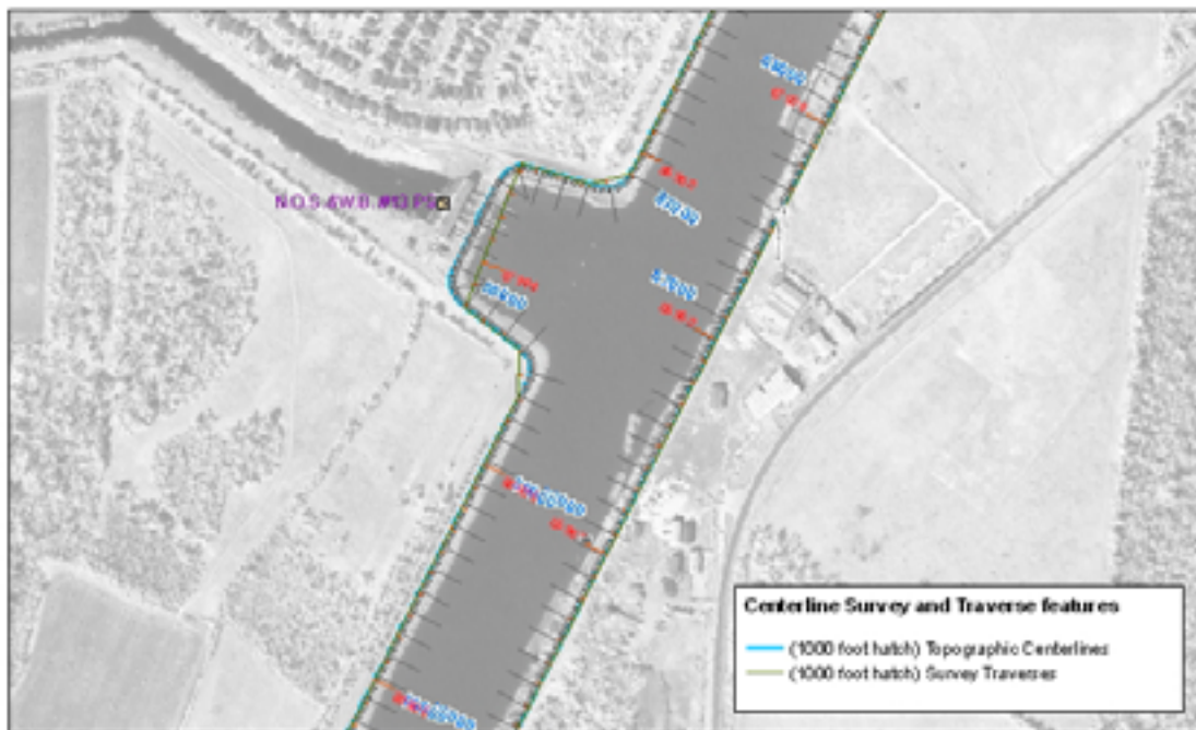
Figure 4 – Example of survey (thick blue line with blue stationing numbers) and traverse (thin green line with red stationing numbers) from a section of the West Bank and Vicinity – Harvey to Algiers levee reach in the New Orleans West Bank hurricane protection system. In this example, the survey and traverse both follow the floodwall that extends back to the pump station structure. Traverse stationing was directly assigned to the survey centerline. Minor angular differences between the traverse and the centerline tend to cancel each other out over the length of the topographic centerline reach.
