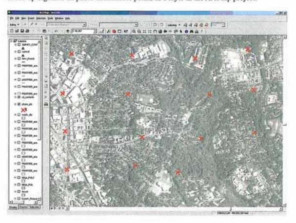
This process took nearly two days to accurately identify each point. Then the points were exported and uploaded to Delorme Street Atlas 2005 software on a Panasonic Toughbook. The field crew was ready to go into the field, equipped with contact prints, field computer and Trimble R8 GPS receivers.
