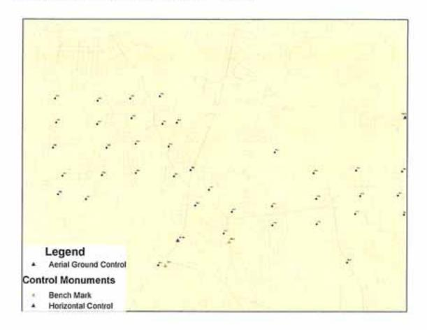
Upon the completion of map compilation of the route, crews took to the field again to provide field edits of the base mapping and obtain attributes on nearly 2500 buildings within the corridor. It is common for field editing to be conducted by visiting a site and marking up a plot of the mapping for said site. Then the marked-up plot is used by someone to make edits in AutoCad to the base map before final delivery and use.
