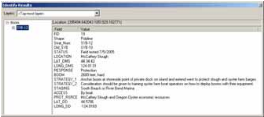
Figure 4. Non-Spatial Attribute Information associated with Strategy Number SY-12 displayed within GIS using Identify Tool.
