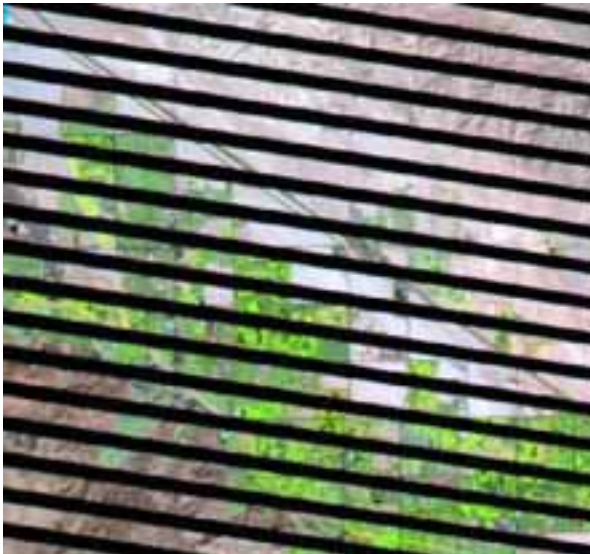
(Figure 2) Example of Landsat 7 TM Imagery with gaps resulting from SLC anomaly (Courtesy USGS/EROS)
