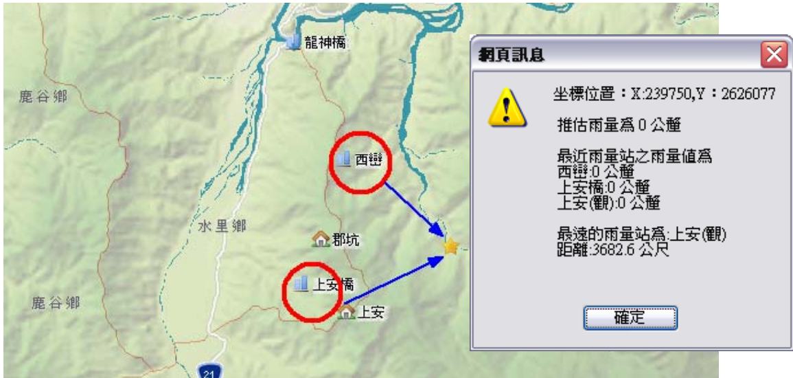
Fig.3 Calculation of rainfall by interpolation from nearby rain gauge stations
