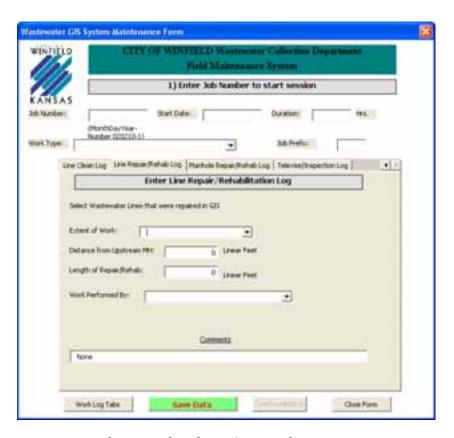
Figure 4: User form interface for gathering information on a wastewater line repair or rehabilitation.
