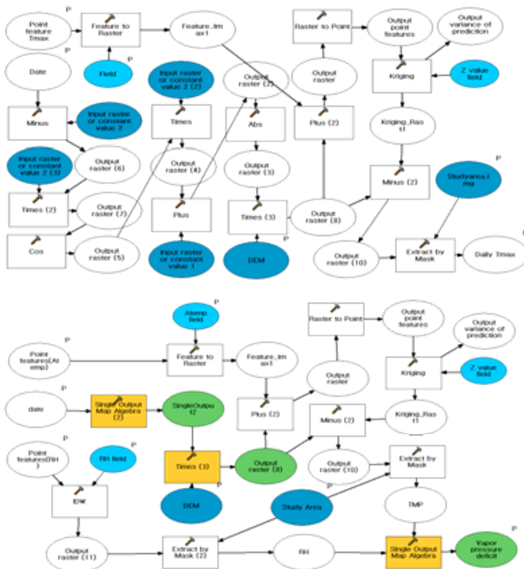
Fig 2. Diagram of absolute lapse rate and vapor pressure deficit calculation using ArcGIS 9.2 model builder
