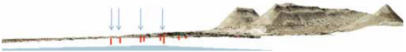
Figure 6G A 3-D perspective view of Dukhan showing selected geotechnical borehole locations (arrows) in relation to development. A GIS development initiative from Qatar Petroleum's Technical Directorate is integrating all geotechnical borehole and trial pits results data to assist in future planning of construction projects.
