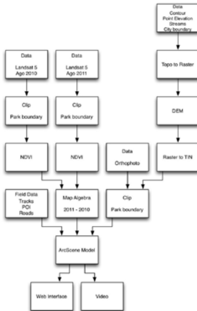
Fig 3: Methodology used, showing the sequence of data preprocessing and NDVI calculation, in parallel with the creation of the 3D model. The integrated results are presented using a Web interface.
