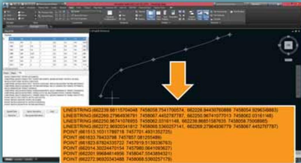
The AutoCAD® geometry can be saved and retrieved as text and the information of various drawings can be combined into the database. The information is organized in SQL Views and can be added to ArcGIS to be shared.
