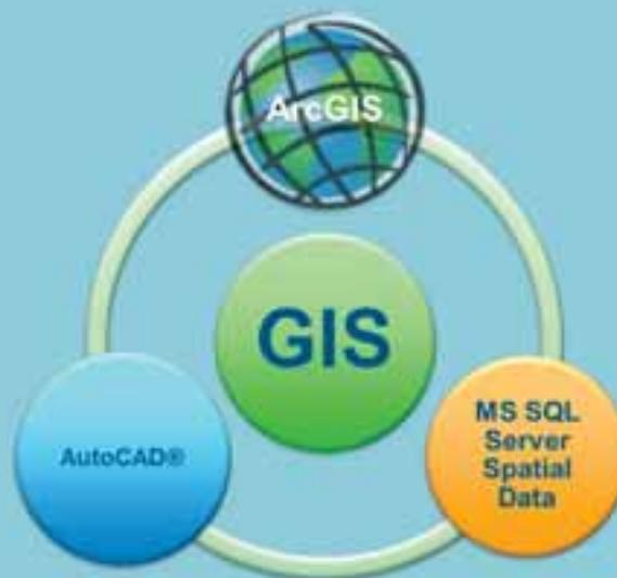
This model allows the engineers to query any layer on the map server and get the results drawn directly into the AutoCAD®'s document. They can edit the drawing and get the information from various sources to compose a new project. Allows them to select the geometry in the drawing and send it as a parameter to query the map server or to perform spatial analysis.
