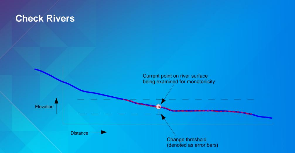
River elevation profile shown above, where red denotes the extent of the river that must be compared with the current surface point (shown as a circle) to establish whether it is part of a monotonic flow
