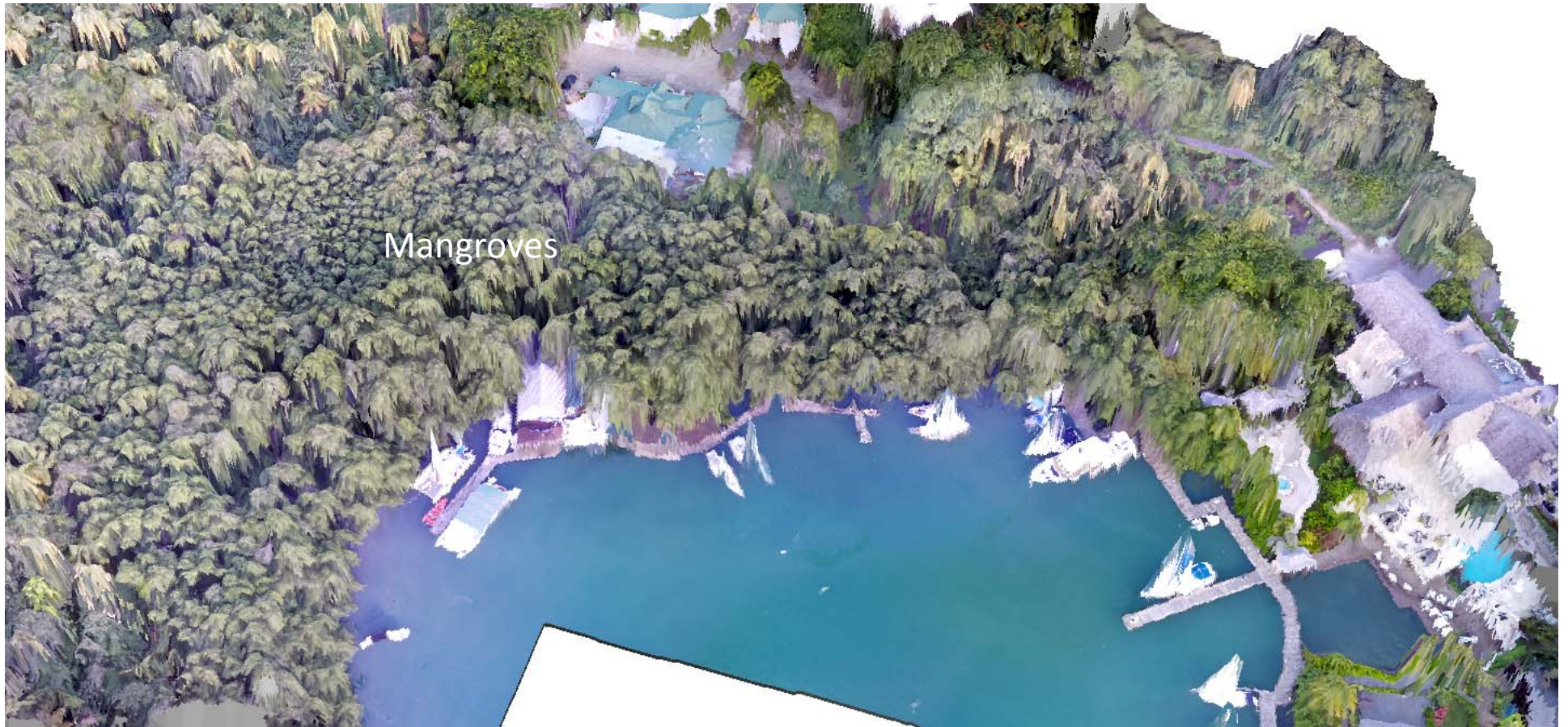
Orthoimagery draped over digital surface model (2cm resolution) created from the stereopair images that were collected on Oct 15 at Marigot Bay.
