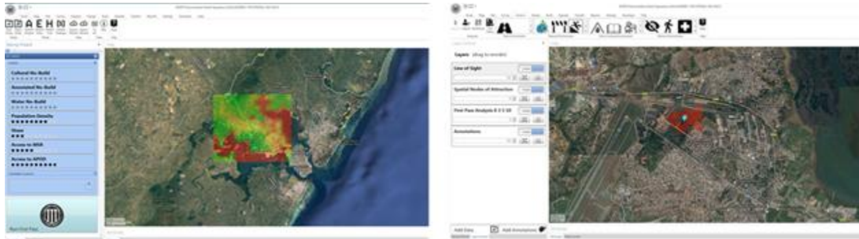
Figure 1 Two screen shots representing the geodesign software, ENSITE. The left demonstrates a the multi-criterion decision analysis run for the area. The right shows a view shed analysis for one base.
