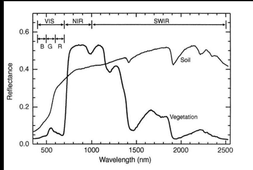
These spectra are used for direct identification of soils/minerals/vegetation and provide information on physical and chemical properties based on wavelength position and shape of absorption features
