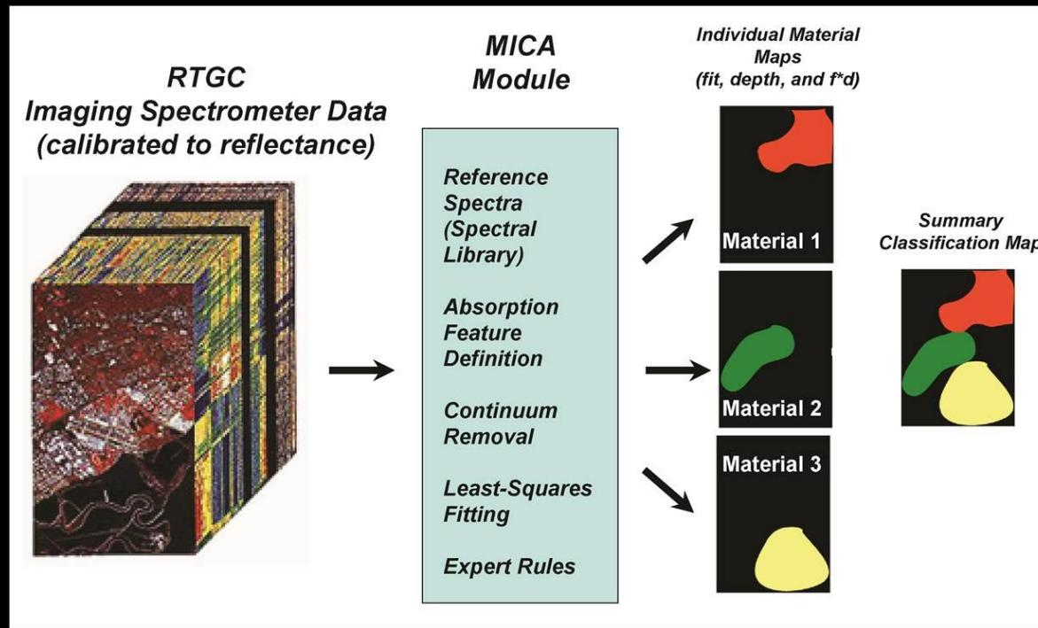
The spectra of the unknown materials are compared with standard library materials as part of the data analysis. The USGS maintains and updates the premier geoscience spectral library. It contains the spectra of hundreds of well-characterized natural and anthropogenic materials. <http://speclab.cr.usgs.gov/spectral.lib06/>
